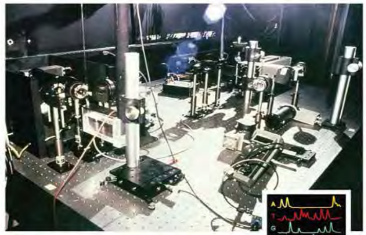
Photo: First automated DNA sequencing machine. Credit: Lloyd Smith.
